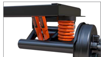
Coil spring with bump stops to prevent harsh 'bottoming out'
